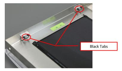
5. Use the narrow walled 3/8" nut driver to secure the four supplied 3/8" hollow nuts to the black UV blocking cover hinge tabs.
